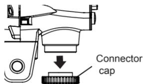
**3** Align the convex part on the strobe's connector with the notch of the sync cord's connector, and then push it straight in
