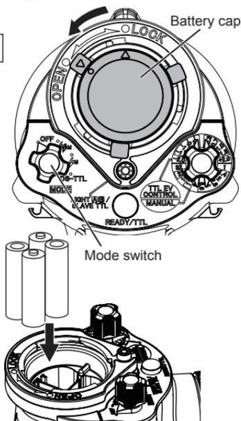
5 Verify that the ○ mark on the battery cap is lined up with the ▽ mark
